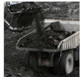
Understanding the properties of a stored material is critical. Some coals, for example, are volatile enough to catch fire during shipping. If uncaught and loaded into a silo this coal can ignite an entire pile.
