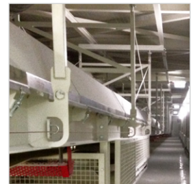
A well ventilated conveying system, designed to reduce dust.
